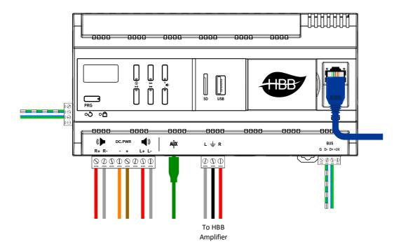
\*\*\* Do not connect more than 1 pair of speakers to the stereo outputs. If you need more speakers you have to add an Amplifier module.
